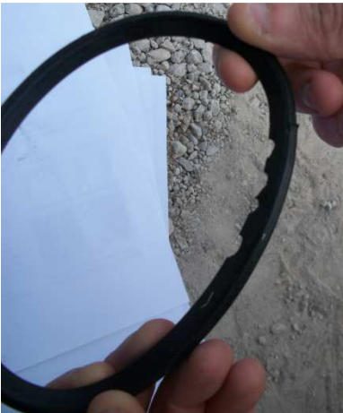
Don't use damaged gasket
